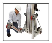
Legs unlock with plunger pin and fold up for storage. Roller wheels under each leg for ease of moving lift in stored position.
