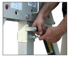
Adjust mast lifting handle with plunger pin to comfortable lifting position
