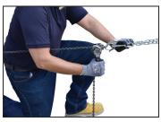
The GH5T comes with chain & ratchet to pull A-Frame legs together.
