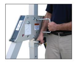
Lift mast and remove quickaction mast locking pin
